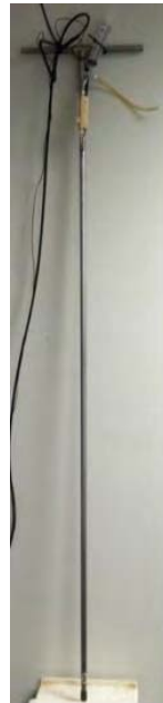
Fabricated depth-specific porewater sampling Device
