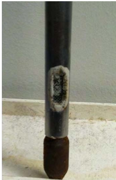
Fabricated depth-specific porewater sampling Device
